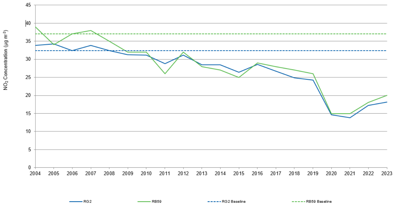
Figure 12 NO2 levels at Horley monitoring stations
