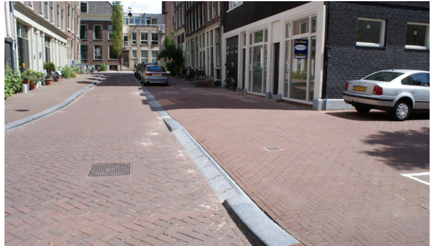
Image 4.4: Example of crossover junction design
