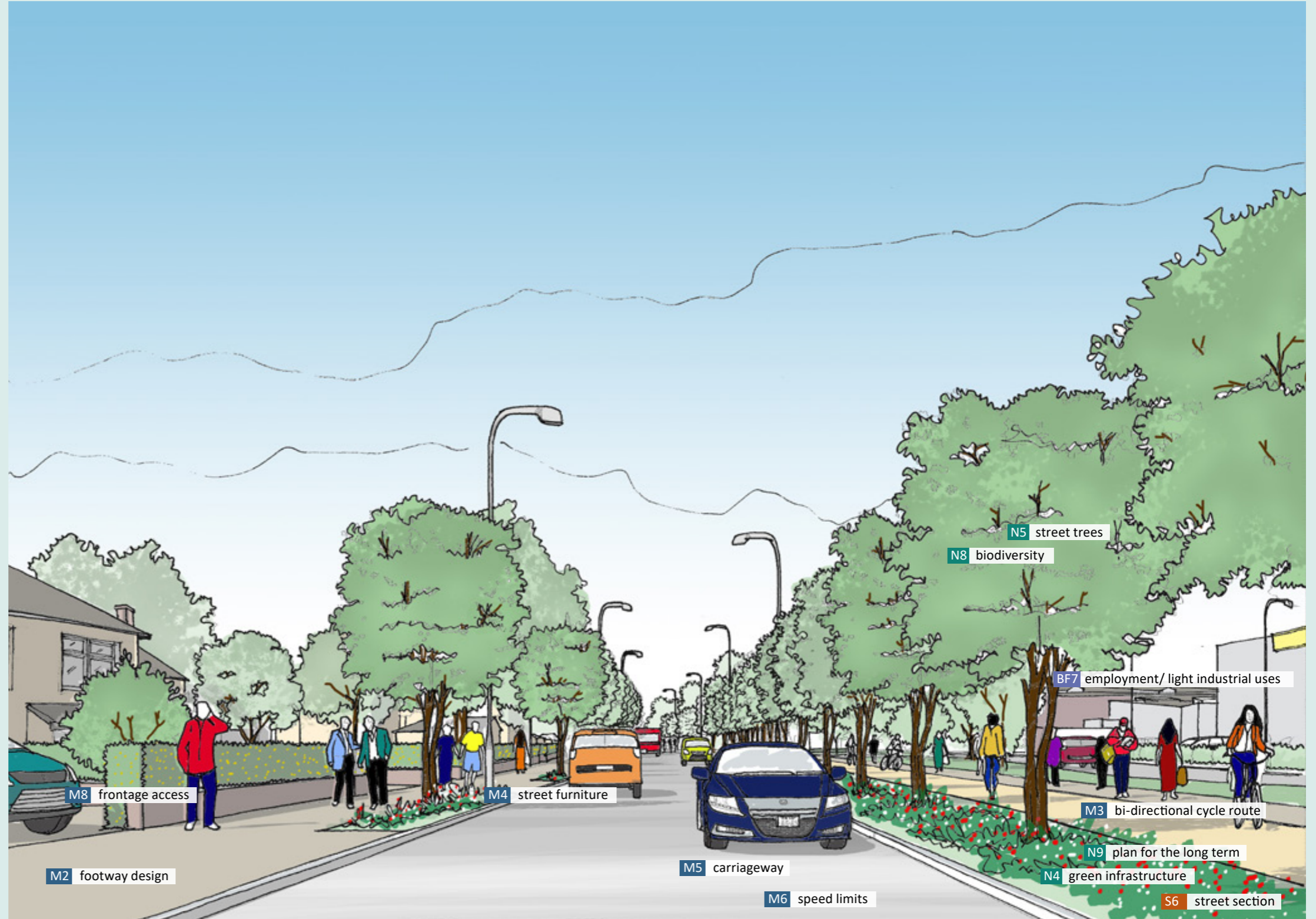
Figure 5.7: Sketch indicating application of the code on the A23 in south Salfords including introduction of street trees and planted verges / raingardens to enhance biodiversity
